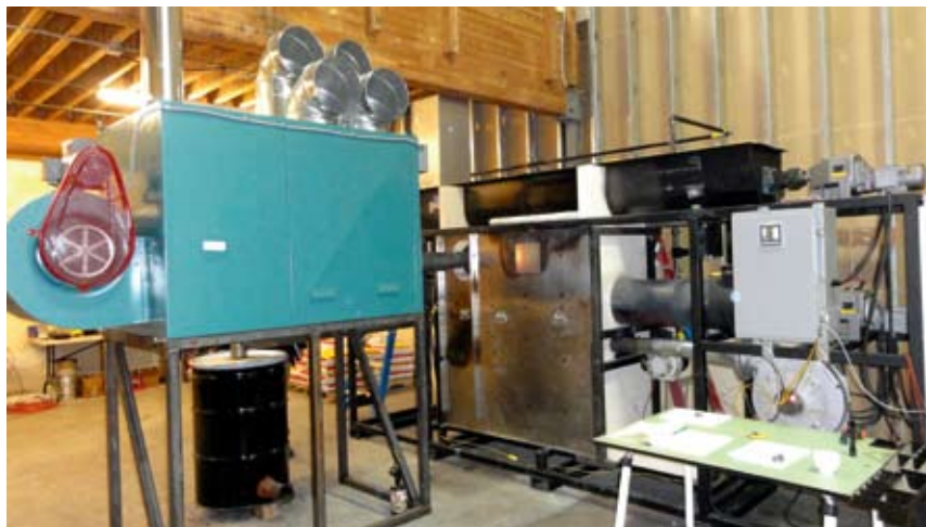
This Whitfield biochar furnace prototype uses pyrolysis to heat a greenhouse and produce biochar from wood pellets.
